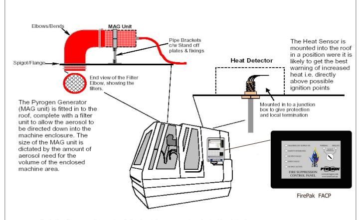
Both the Pyrogen Generator & the heat Sensor are terminated back to the FirePak FACP Control Panel, which once a signal is received from the sensor, will activate Alarms/Sounders, Main fire control systems & the Pyrogen Generator.
